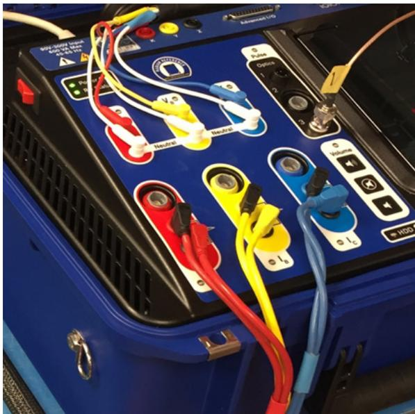
3. Connect the voltage cables to the RW as shown, with the colored cables corresponding to each phase:
